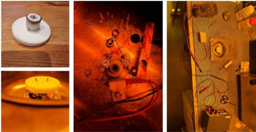
Figure 7.1. Photographs of the custom-built electric-field-assisted spin-coating setup. (Left) Teflon rotation chuck with embedded electrode contacts. (Center) Rolling contact mechanism with miniature ball bearings integrated into the spinner base. (Right) Complete spin-coating workstation with DC power supply and current-measurement circuit.
