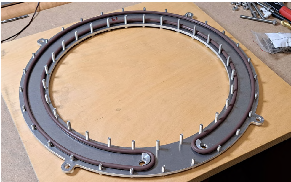
Figure 5.42: Photograph of an aluminium carcass ring used in the MOT coil assembly. The Viton O-ring seal is visible, forming the cooling channel between the paired rings. Mounting brackets for fixing the carcass to the UHV chamber are also visible.
