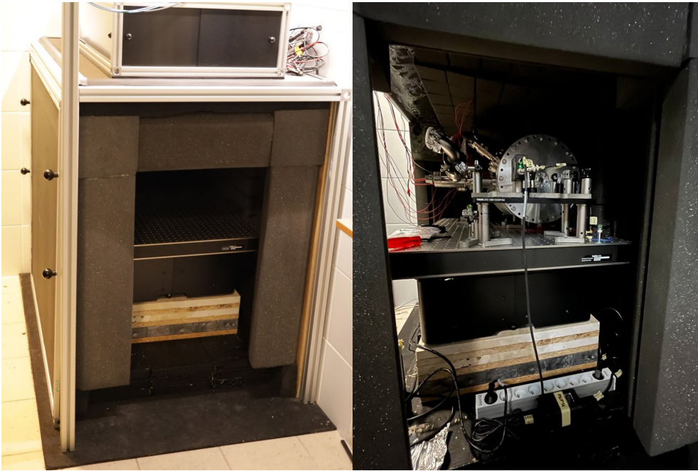
Figure 5.12: Photos of the acoustic isolation system before (left) and after (right) the installation of the optical cavity and associated optics. The vacuum system is mounted on a passive anti-vibration platform placed atop a custom-designed vibration-damping pillar composed of layered construction materials. The pillar lies on a 1 cm-thick dense rubber damping mat and incorporates successive layers of concrete, MDF, lead, and marble to attenuate mechanical disturbances. Ceramic slabs with Viton half-balls (not seen in the picture) are placed between the anti-vibration platform and the optical breadboard to provide further mechanical decoupling. The entire setup is enclosed in a cuboid acoustic housing, constructed from 45 mm aluminium profiles and OSB panels, with internal and external acoustic foams for suppression of ambient acoustic noise.
