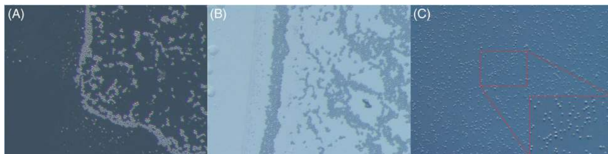
FIGURE 4 Optical microscope images for stationary phase slurries of Diol-P-C10 in methanol (A), isopropanol (B), and acetonitrile (C). The differences in the shading of the images are due to differences in the refractive indices of the solvents, so the light intensity during the observations varied. The absence of a photo for the chloroform slurry is due to the fast evaporation of the solvent
