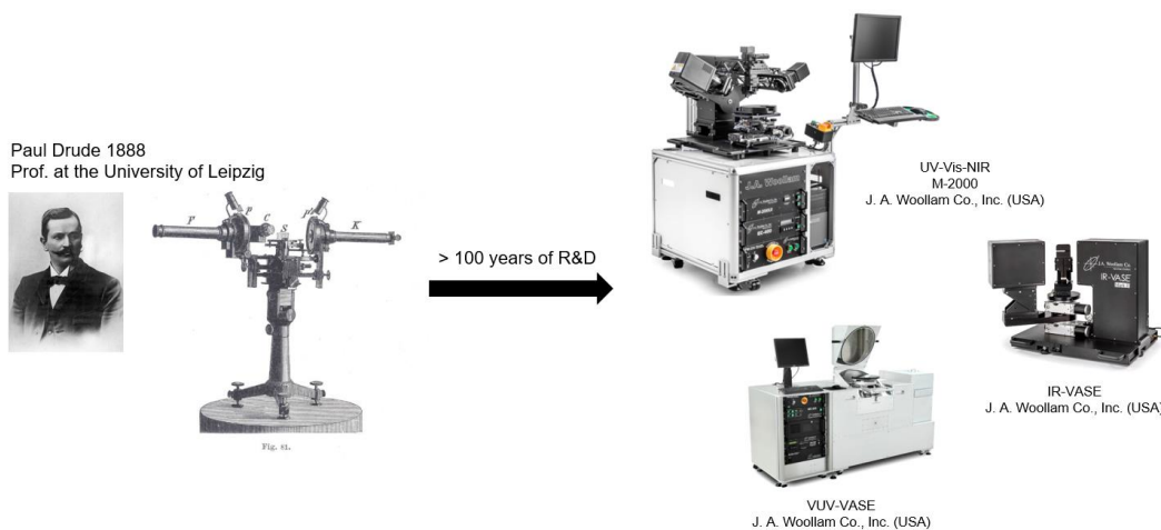
Figure 2 (left) A photograph of Paul Drude together with his original ellipsometer used at the University of Leipzig (right) examples of ellipsometers currently used to study optical properties of matter at a variety of wavelength ranges
