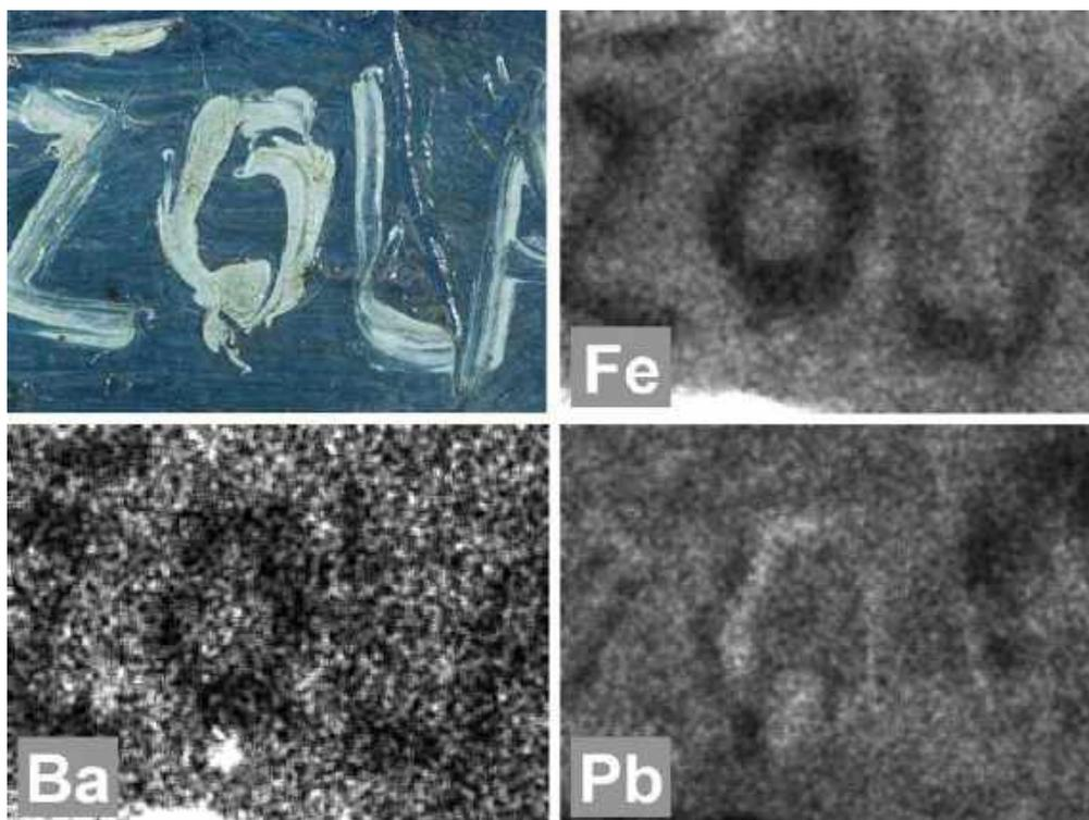
**Fig. 12** Close-up of the detail of the blue street sign from *Zuo La Lu* and MA-XRF maps. The distribution of the three main elements, Fe, Ba, Pb, is shown. Fe-signal relates to the Prussian blue later identified with SEM–EDS and PLM. The greyscale corresponds to the intensity of the signal of each element: white equals high intensity, black means low intensity
