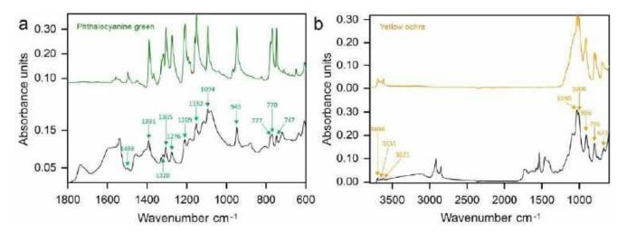
**Figure 13.** (a) ATR–FTIR spectra of the green paint of sample 4 extracted from *Mount Huangshan* (1983), with labelled marker peaks of phthalocyanine green and reference spectra of the same pigment. (b) ATR–FTIR spectra of the green paint of sample 4 extracted from *Mount Huangshan* (1986), with labelled marker peaks of yellow ochre admixture and reference spectra of the same pigment.
