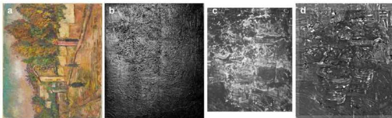
**Figure 20.** Images of *Autumn colours* rotated at 90° anticlockwise and photographed in: (a) VIS; (b) RTI; and (c) transmitted NIR executed with camera facing the back of the painting, then cropped to remove the strainer bars, inverted horizontally, and reproduced with the same relative scale; (d) XRR. The images revealed paint features of hidden still life painting with plants in the flowerpots.
