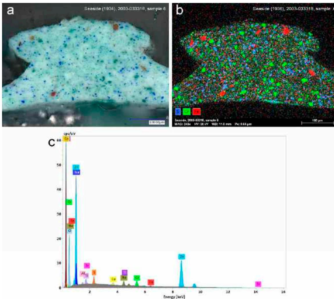
**Figure 8.** Microscopy image (a), corresponding SEM-EDS elemental map (b) and SEM-EDS spectra (c) of sample 6, extracted from *Seaside*, 1936. The SEM-EDS analyses show the distribution of S elements relating to ultramarine, Cr relating to viridian and Fe attributing to yellow iron-containing earth in the paint sample.
