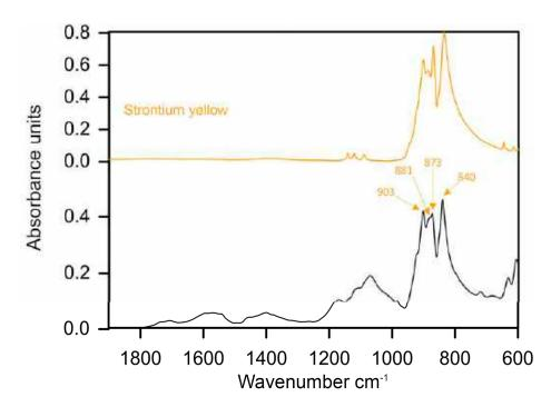
**Figure 11.** ATR–FTIR spectra obtained from the green paint of sample 10, extracted from *Backyard*, 1934 with labelled marker peaks of strontium yellow and reference spectra of the same pigment.
