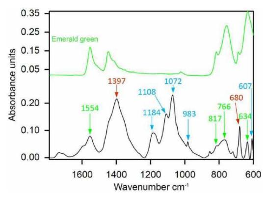
**Figure 6.** ATR-FTIR spectra of the green paint of sample 4 extracted from Nude (1927) with labelled (green) marker peaks of emerald green and reference spectra of the same pigment. Bands labelled in red indicate lead white and bands labelled in blue refer to lithopone. However, band 634 cm<sup>-1</sup> is indicative of both emerald green and lithopone.
