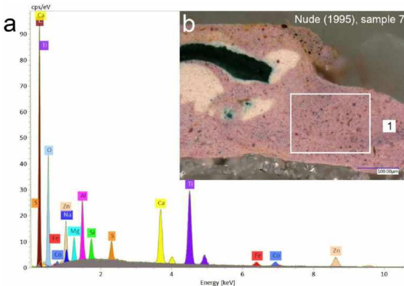
**Figure 11.** (a) SEM-EDS spectra of the pink paint from layer 1 of sample 7 extracted from *Nude* (1995); (b) optical microscopy image of the cross-section of the sample at 200× magnification, with marked area of analyses.
