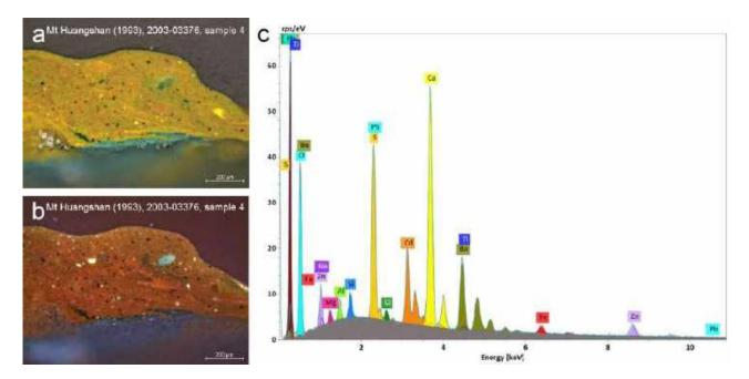
**Figure 12.** Optical microscopy images of the paint cross-section of sample 4, extracted from *Mount Huangshan*, 1993, photographed in: (a) VIS and (b) UV. The corresponding SEM-EDS spectra of the yellow paint (c). Red fluorescence of yellow paint and strong Cd and S signals combined with Ba and Zn suggests the use of cadmium yellow or cadmopone or zinc-modified light cadmium yellow.
