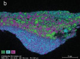
**Figure 10.** Microscopy image (a) and corresponding SEM-EDS mapping of sample c24 of *Climbing the hill* (b). The SEM-EDS mapping shows the distribution of chromium (Cr), zinc (Zn) and barium (Ba) in the paint sample.
