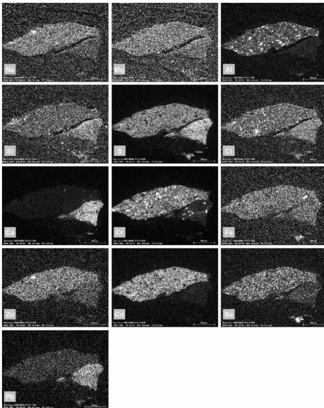
**Fig. 20** SEM-EDS maps showing the distribution of the detected elements in sample 8 from *Zuo La Lu*. The greyscale corresponds to the intensity of the signal of each element: white equals high intensity, black means low intensity. Cadmium, which was assigned to cadmium yellow, is confined only to the upper layer while the second layer is characterised mainly by Ca, Pb and Cr
