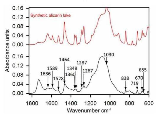
**Figure 10.** ATR-FTIR spectra of the red paint of sample 2 extracted from *Nude* (1992), with labelled marker peaks of synthetic alizarin lake and reference spectra of the same pigment.
