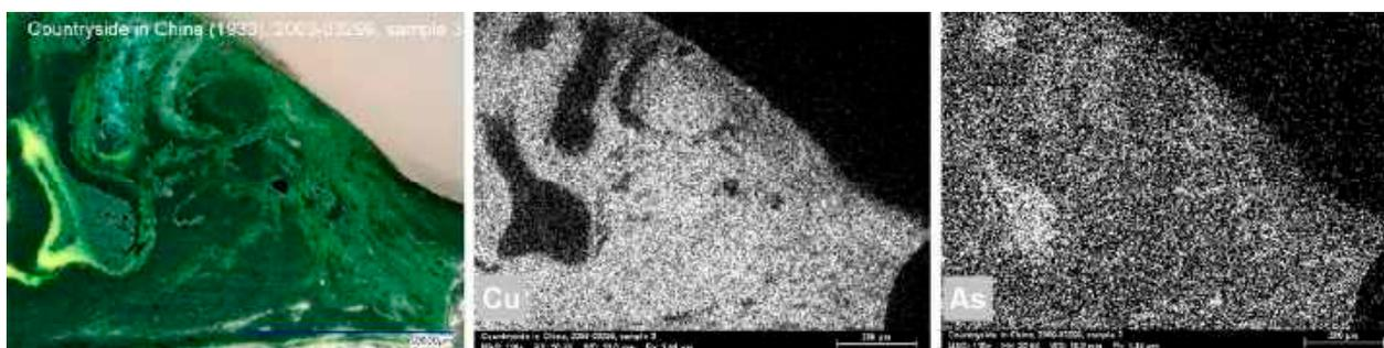
**Figure 10.** Optical microscopy image of the paint cross-section of sample 3 obtained from *Countryside in China*, 1933 and captured at 100× magnification (top-left), followed by SEM-EDS elemental distribution maps. The intensity of the signal of each element is represented by a range of grey tones: white represents high intensity and black represents low intensity. A concomitant presence of highly intensive copper and arsenic signals suggests the use of emerald green.
