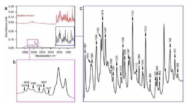
**Figure 12.** (a) ATR-FTIR spectra of the pink paint of sample 2 extracted from *Two nudes* (1996), with labelled marker peaks of naphthol red AS-D and reference spectra of the same pigment; (b) a scale expansion of the spectra of the sample from 2700 to  $3300 \, \text{cm}^{-1}$ ; (c) a scale expansion of the spectra of the sample from 600 to  $1700 \, \text{cm}^{-1}$ .
