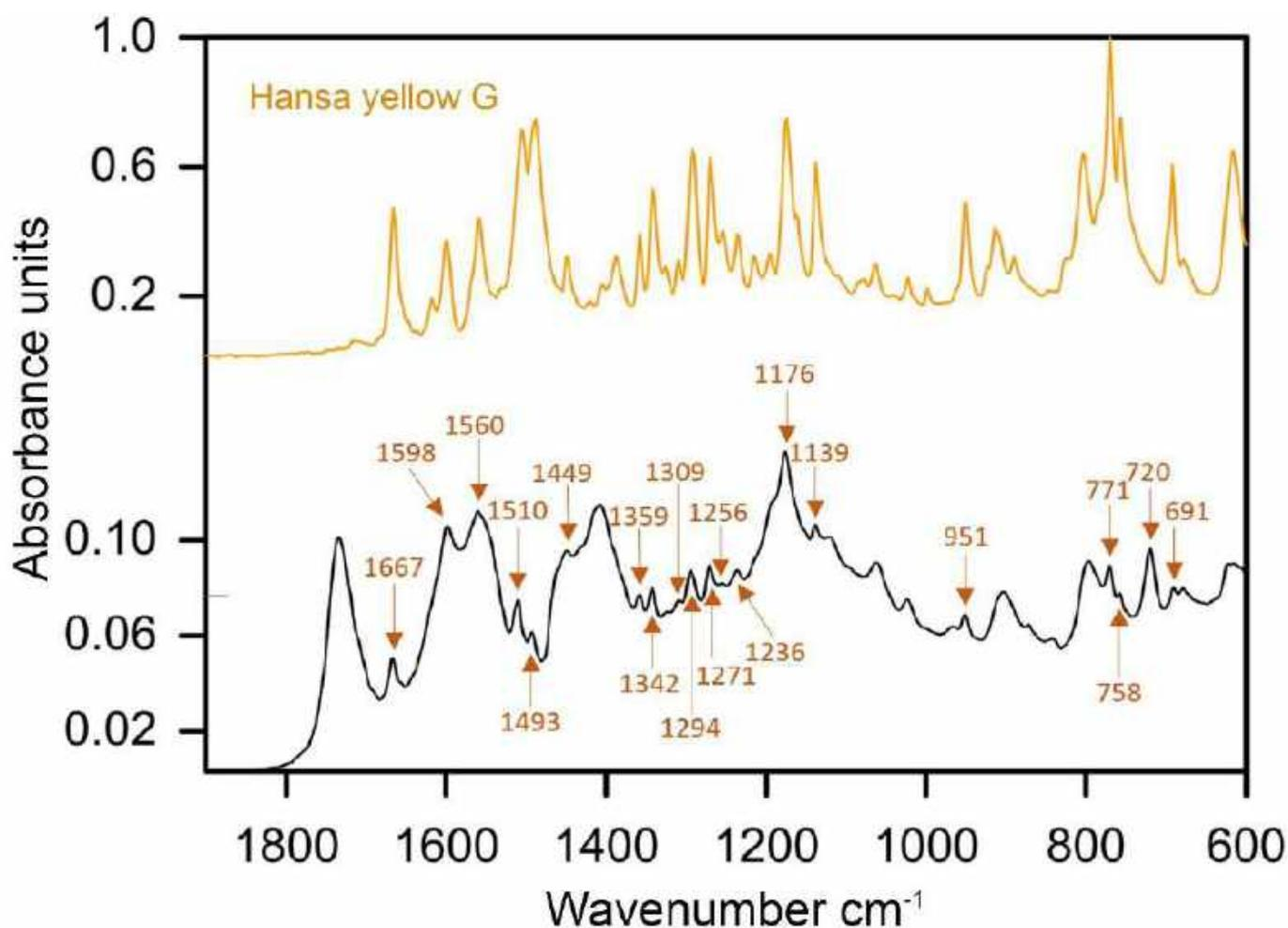
**Figure 14.** ATR-FTIR spectra of the green paint of sample 3 extracted from *Mount Huangshan* (1995), with labelled marker peaks of Hansa yellow G and reference spectra of the same pigment.
