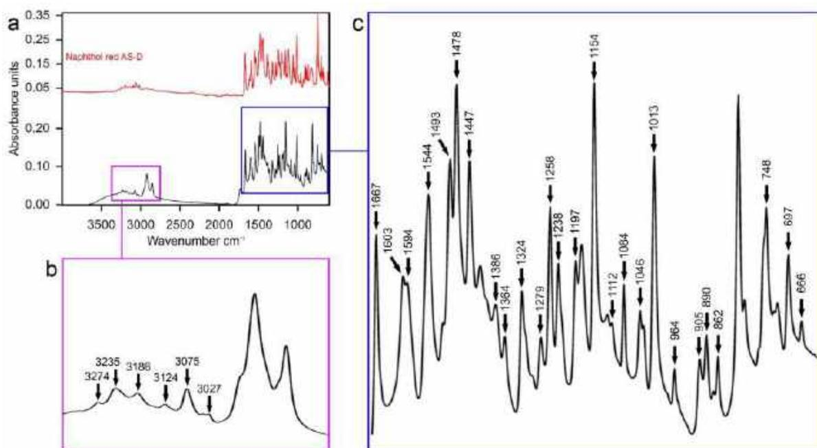
**Figure 12.** (a) ATR-FTIR spectra of the pink paint of sample 2 extracted from *Two nudes* (1996), with labelled marker peaks of naphthol red AS-D and reference spectra of the same pigment; (b) a scale expansion of the spectra of the sample from 2700 to  $3300\text{ cm}^{-1}$ ; (c) a scale expansion of the spectra of the sample from 600 to  $1700\text{ cm}^{-1}$ .
