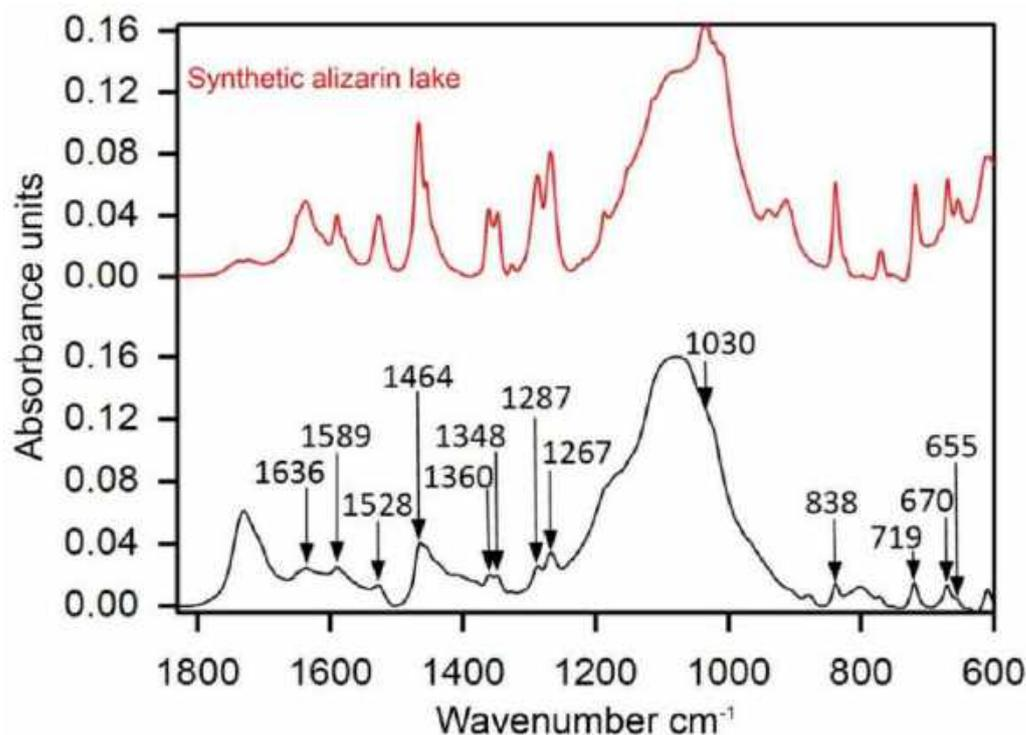
**Figure 10.** ATR-FTIR spectra of the red paint of sample 2 extracted from *Nude* (1992), with labelled marker peaks of synthetic alizarin lake and reference spectra of the same pigment.
