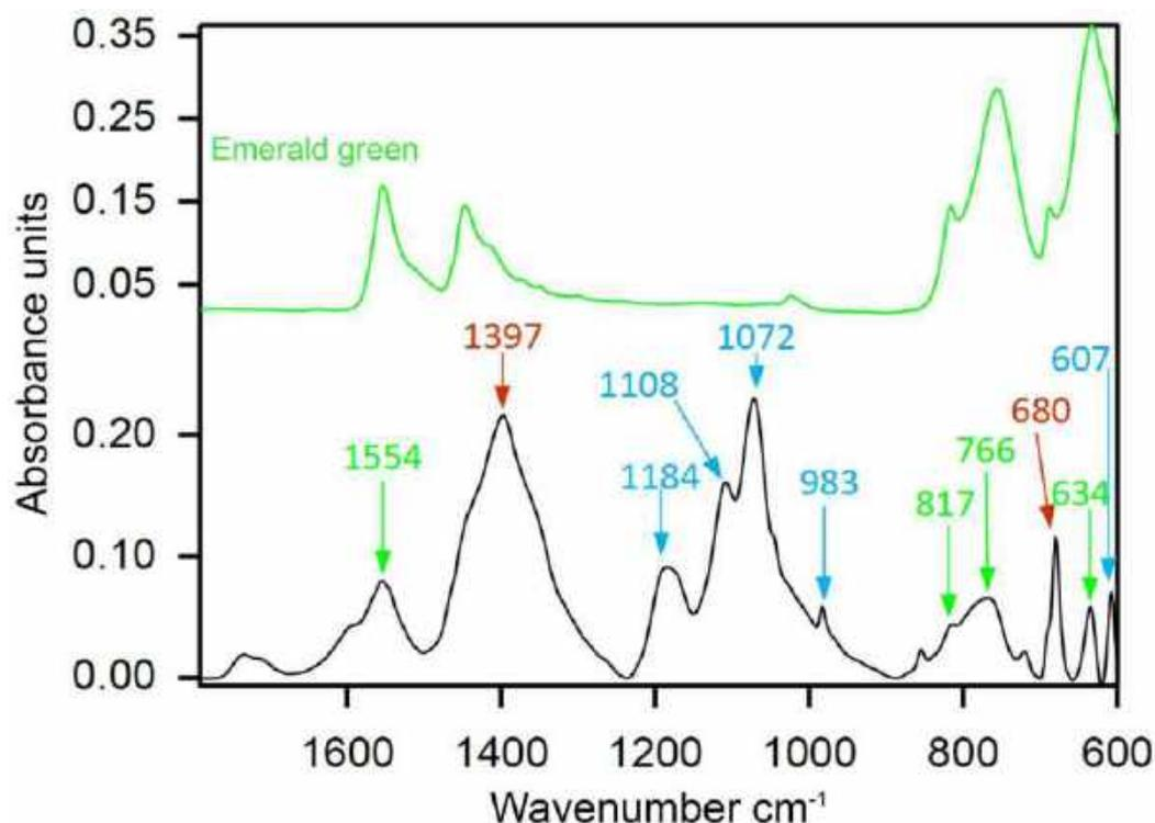
**Figure 6.** ATR-FTIR spectra of the green paint of sample 4 extracted from *Nude* (1927) with labelled (green) marker peaks of emerald green and reference spectra of the same pigment. Bands labelled in red indicate lead white and bands labelled in blue refer to lithopone. However, band  $634\text{ cm}^{-1}$  is indicative of both emerald green and lithopone.
