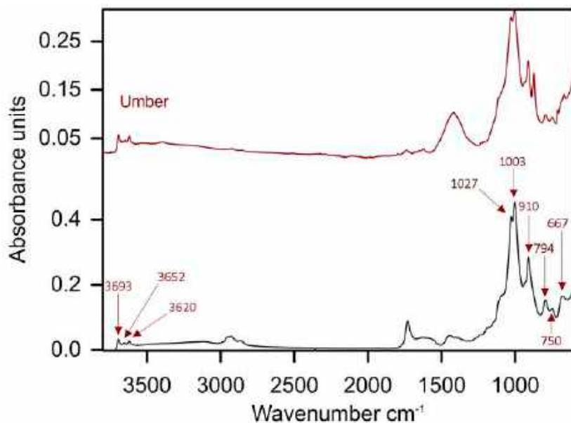
**Figure 13.** ATR-FTIR spectra of the brown paint of sample 11, extracted from *Working at the fields*, 1933, with labelled marker peaks of umber and reference spectra of the same pigment.
