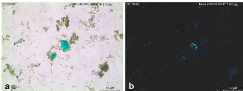
**Fig. 21** Viridian particles from sample 7 taken from green curtain behind the model from *Nude*, photographed in transmitted polarized (a) and between crossed polars (b)
