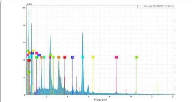
**Fig. 16** SEM–EDS quantitative elemental analysis of the top green layer in sample 8 from *Zuo La Lu*. The spectra indicates elements that were assigned to viridian, ultramarine, Prussian blue, lead white and cadmium yellow. Cadmium yellow is characterised by strong Cd- and S-signals. The findings were correlated with PLM observations
