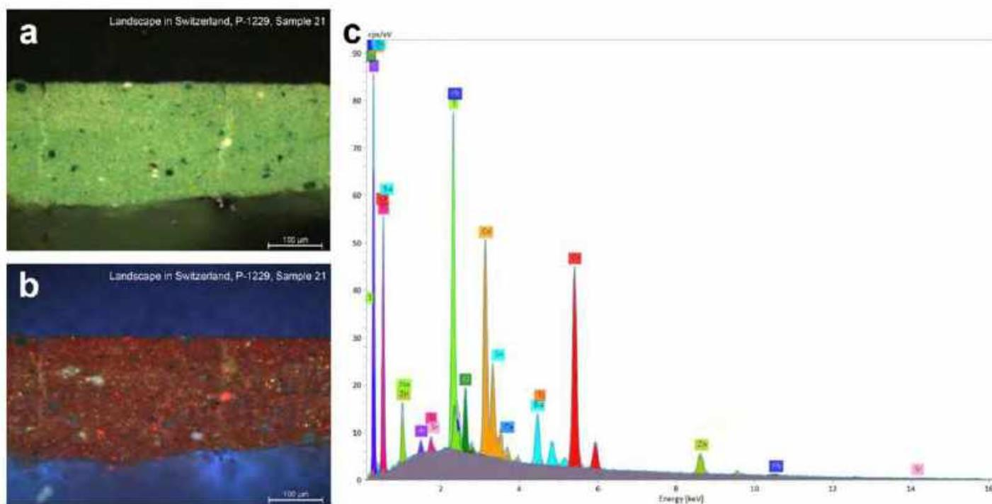
**Figure 6.** Microscopy images of the cross-section of sample 21, extracted from *Landscape in Switzerland*, photographed in: (a) VIS; (b) UV. The corresponding SEM-EDS spectra of the green paint are seen in (c). Red fluorescence of yellow particles and a strong Cd-signal suggested the presence of cadmium yellow.
