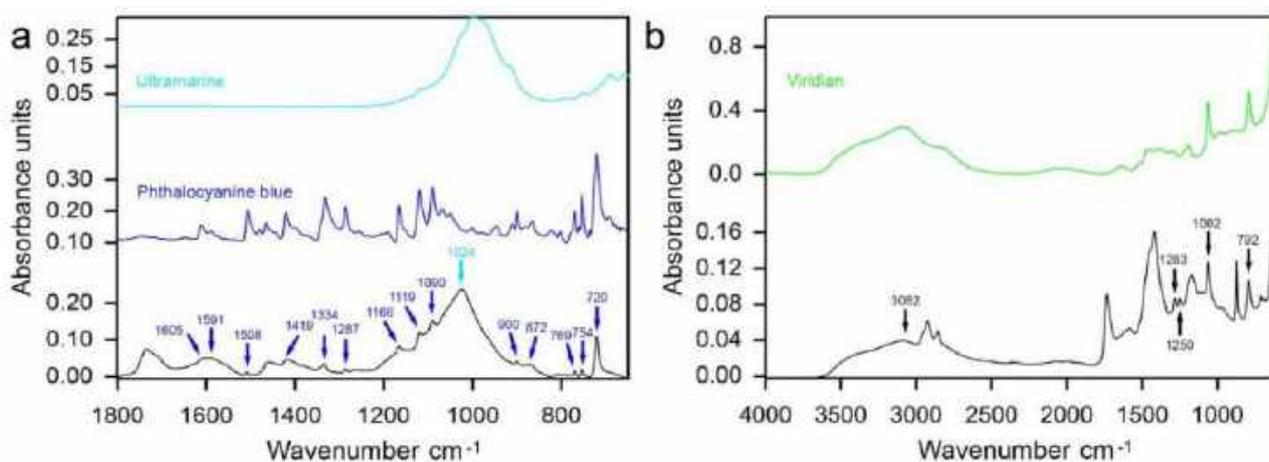
**Figure 14.** (a) ATR-FTIR spectra of the black paint of sample 13 extracted from *Beauties at rest II* (1998), with labelled (dark blue) marker peaks of phthalocyanine blue and ultramarine (light blue) and reference spectra of the same pigments; (b) ATR-FTIR spectra of the green paint of sample 3 extracted from *Beauties at rest II* (1998), with labelled marker peaks of viridian and reference spectra of the same pigment.
