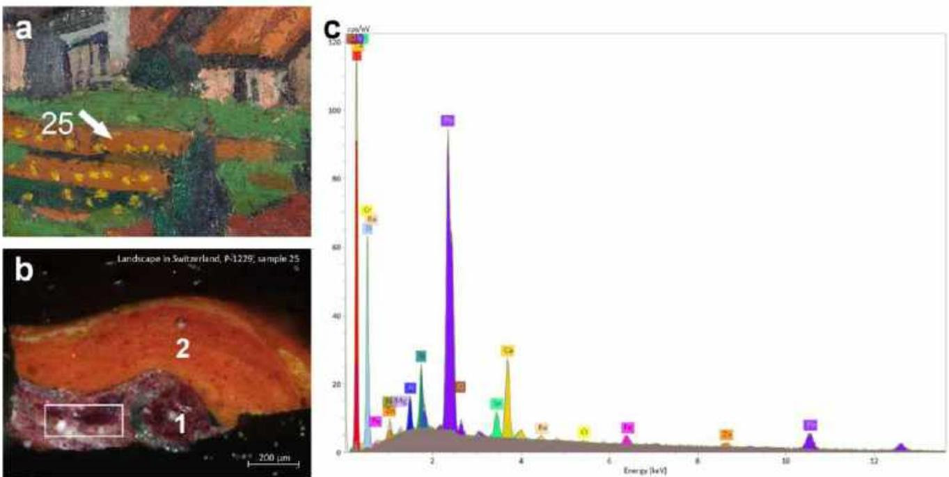
**Figure 11.** (a) Detail of *Landscape in Switzerland*, showing the sampling spot; (b) microscopy image of the cross-section of sample 25 with the marked area of SEM-EDS elemental analyses; (c) corresponding SEM-EDS spectra of the analysed area from layer 1, indicating a strong Sn-signal from the tin substrate of organic red.
