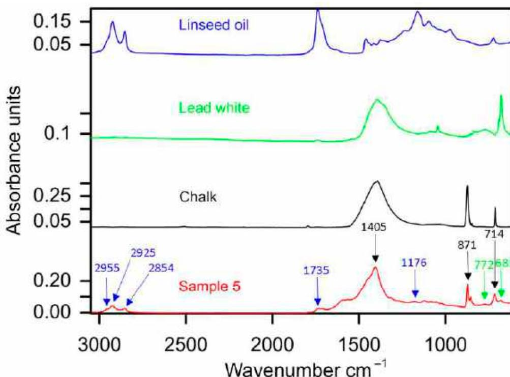
**Figure 6.** ATR-FTIR spectra of the white ground layer of sample 5 extracted from *Nude*, 1927, with labelled marker peaks of chalk (black), lead white (green), oil (blue) and reference spectra of the same compounds.
