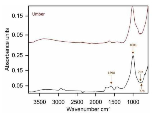
**Figure 11.** ATR–FTIR spectra of the brown paint of sample 4 extracted from *Mount Huangshan* (1987), with labelled marker peaks of umber and reference spectra of the same pigment.
