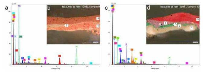
**Figure 13.** (a) SEM-EDS spectra of the orange paint from layer 3 of sample 9 extracted from *Beauties at rest II* (1998); (b) corresponding optical microscopy image of the cross-section of the sample at  $200 \times$  magnification; (c) SEM-EDS spectra of the red paint from layer 5 of sample 10 extracted from *Beauties at rest* (1998); (d) corresponding optical microscopy image of the cross-section of the sample at  $200 \times$  magnification.
