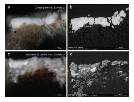
**Figure 8.** Microscopy and corresponding backscattered electron images (BSE) of cross-sections showing: the homogenous structure of ground layer extracted from: *Climbing the hill* (a, b); structure of the ground layer characterised by large particles of chalk (visualised in dark grey in BSE image) from *View from St. John's Fort* (c, d).
