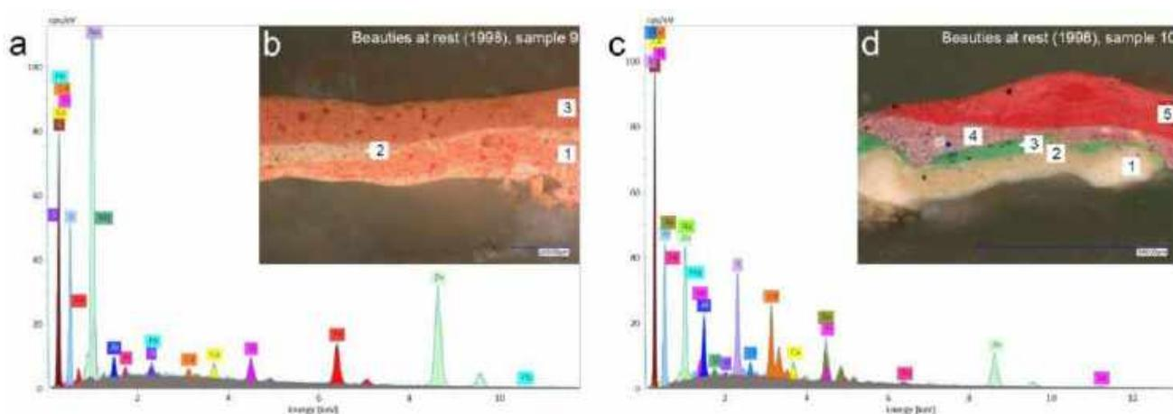
**Figure 13.** (a) SEM-EDS spectra of the orange paint from layer 3 of sample 9 extracted from *Beauties at rest II* (1998); (b) corresponding optical microscopy image of the cross-section of the sample at  $200\times$  magnification; (c) SEM-EDS spectra of the red paint from layer 5 of sample 10 extracted from *Beauties at rest II* (1998); (d) corresponding optical microscopy image of the cross-section of the sample at  $200\times$  magnification.
