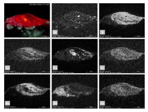
**Fig. 6.** Microscopy image of the cross-section of sample 21, photographed in visible light, and SEM-EDS maps showing the distribution of the detected elements. The greyscale corresponds to the intensity of the signal of each element: white equals high intensity, black means low intensity. A high concentration of Sn relates to the presence of a tin-based substrate in the paint
