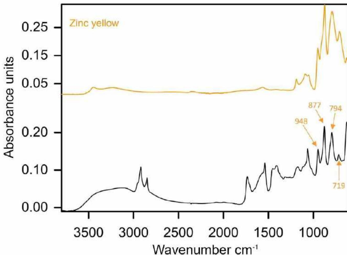
**Figure 15.** ATR-FTIR spectra of the green paint of sample 1 extracted from *Mountain* (1977), with labelled marker peaks of zinc yellow admixture and reference spectra of the same pigment.
