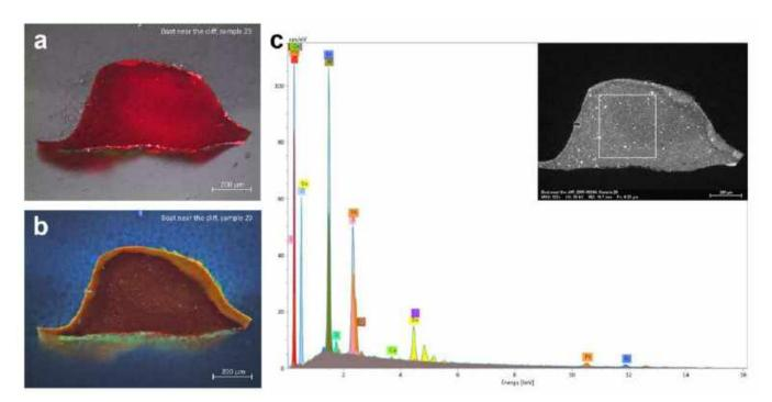
**Figure 12.** Microscopy image of the cross-section of sample 29 extracted from *Boat near the cliff* photographed in: (a) VIS; (b) UV. SEM-EDS spectra of the sample and inset backscattered electron (BSE) image with marked area of analyses (c). The spectra shows Br peaks which could be indicative of geranium lake, as well as Pb, Ba, Al, and S, which can be assigned to lead white and barium white extender and/or Pb- or Al-based substrate.
