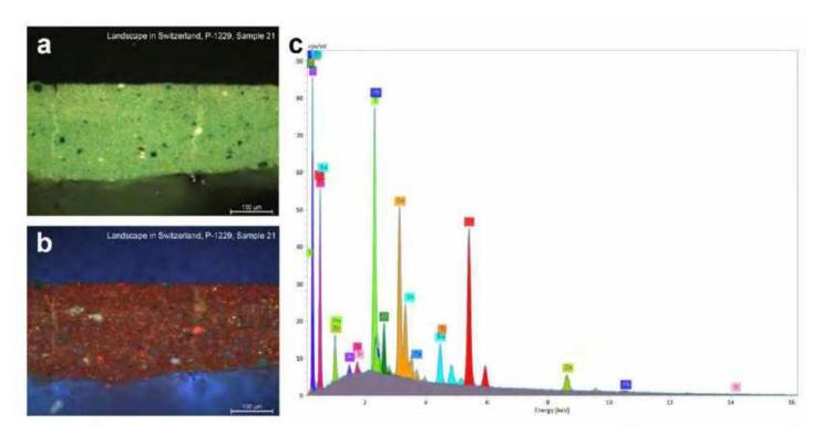
**Figure 6.** Microscopy images of the cross-section of sample 21, extracted from *Landscape in Switzerland*, photographed in: (a) VIS; (b) UV. The corresponding SEM-EDS spectra of the green paint are seen in (c). Red fluorescence of yellow particles and a strong Cd-signal suggested the presence of cadmium yellow.
