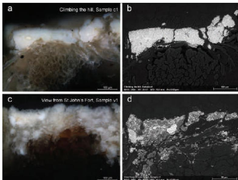
**Figure 8.** Microscopy and corresponding backscattered electron images (BSE) of cross-sections showing: the homogenous structure of ground layer extracted from: *Climbing the hill* (a, b); structure of the ground layer characterised by large particles of chalk (visualised in dark grey in BSE image) from *View from St. John's Fort* (c, d).
