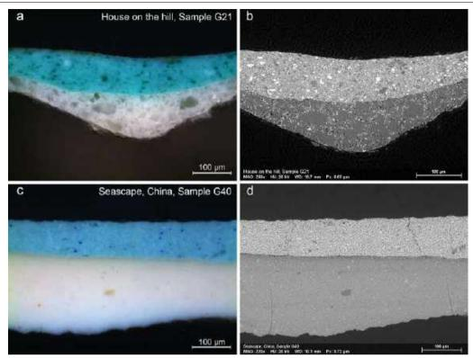
Fig. 13 Microscopy and relevant backscattered electron images (BSE) of cross-sections with ground extracted from the Shanghai paintings. The images show different types of identified grounds: **a**, **b** ground type 1 with large particles of chalk (grey); **c**, **d** ground type 2 with homogenous structure
