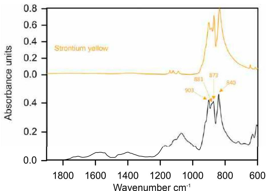
**Figure 11.** ATR-FTIR spectra obtained from the green paint of sample 10, extracted from *Backyard*, 1934 with labelled marker peaks of strontium yellow and reference spectra of the same pigment.
