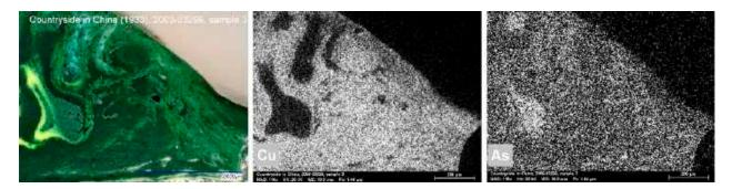
**Figure 10.** Optical microscopy image of the paint cross-section of sample 3 obtained from *Countryside in China*, 1933 and captured at  $100 \times$  magnification (top-left), followed by SEM-EDS elemental distribution maps. The intensity of the signal of each element is represented by a range of grey tones: white represents high intensity and black represents low intensity. A concomitant presence of highly intensive copper and arsenic signals suggests the use of emerald green.
