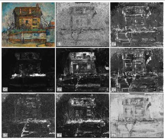
**Fig. 4** Visible light image and MA-XRF maps of *Zuo La Lu* showing the distribution of the detected elements. The greyscale corresponds to the intensity of the signal of each element; white equals high intensity, black means low intensity. Distribution maps of Ca, Zn and Pb reveal the hidden composition rotated at 90° anticlockwise
