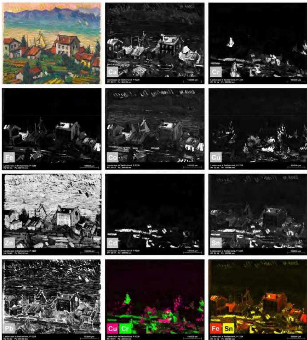
**Figure 4.** Visible light image and MA-XRF maps of *Landscape in Switzerland*, showing the distribution of the major elements. The greyscale corresponds to the intensity of the signal of each element: white equals high intensity, black means low intensity. The colour maps combine distribution of Cu- and Cr-based pigments and Fe- and Sn-based pigments.
