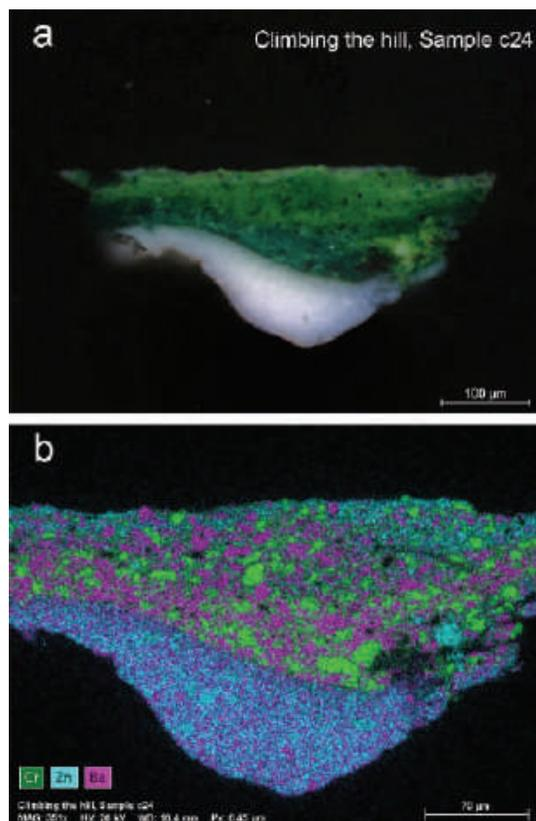
**Figure 10.** Microscopy image (a) and corresponding SEM-EDS mapping of sample c24 of *Climbing the hill* (b). The SEM-EDS mapping shows the distribution of chromium (Cr), zinc (Zn) and barium (Ba) in the paint sample.
