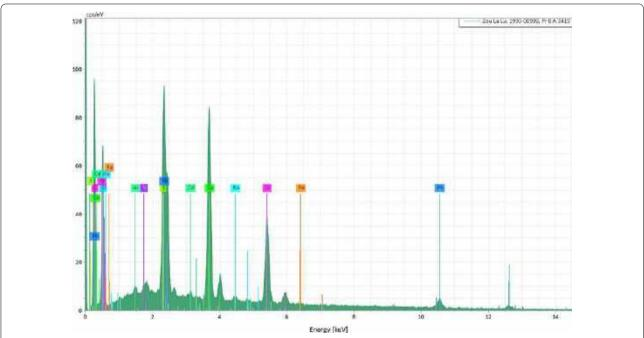
**Fig. 19** SEM-EDS quantitative elemental analysis of green cluster in sample 8, layer 2 from Zuo La Lu. The green paint probably contains Cr-based green and yellow pigments with possible extenders. The weak Cd-signal indicates a trace amount of cadmium yellow
