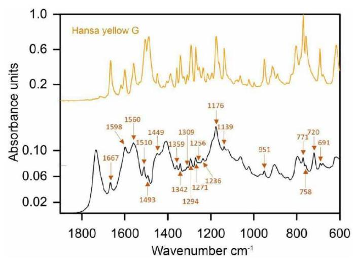
**Figure 14.** ATR–FTIR spectra of the green paint of sample 3 extracted from *Mount Huangshan* (1995), with labelled marker peaks of Hansa yellow G and reference spectra of the same pigment.
