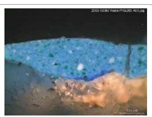
**Fig. 15** Cross-section of sample 9 from *Nude*. The image shows that the blue paint was laid directly on the ground layer, thus suggesting that it may relate to the previous paint scheme
