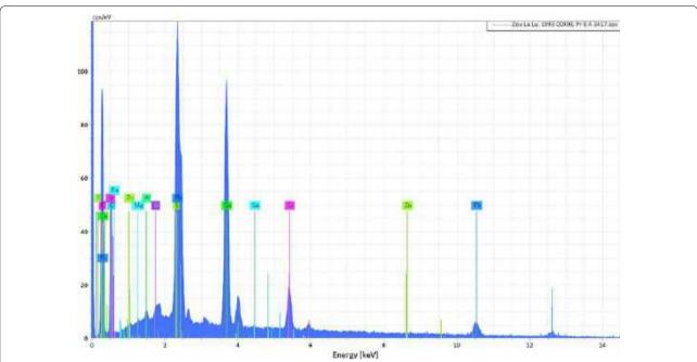
**Fig. 18** SEM-EDS quantitative elemental analysis of yellow cluster in sample 8, layer 2 from *Zuo La Lu*. Cr-containing pigment with possible extenders can be attributed to the yellow paint
