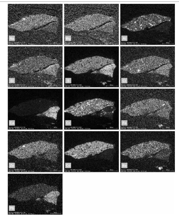
**Fig. 20** SEM-EDS maps showing the distribution of the detected elements in sample 8 from *Zuo La Lu*. The greyscale corresponds to the intensity of the signal of each element: white equals high intensity, black means low intensity. Cadmium, which was assigned to cadmium yellow, is confined only to the upper layer while the second layer is characterised mainly by Ca, Pb and Cr
