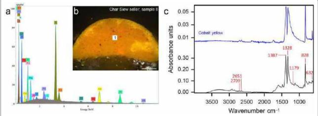
**Fig. 15 a** SEM–EDS spectra of the yellow paint of sample 6 extracted from *Char Siew seller*; **b** optical microscopy image of the cross-section of the sample; **c** corresponding ATR-FTIR spectra of the yellow paint with labelled marker peaks of cobalt yellow and reference spectra of the same pigment
