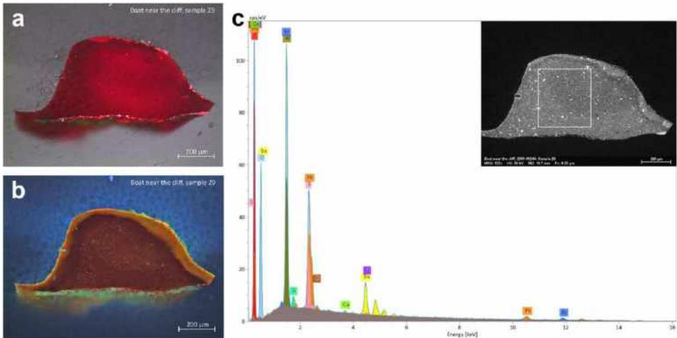
**Figure 12.** Microscopy image of the cross-section of sample 29 extracted from *Boat near the cliff* photographed in: (a) VIS; (b) UV. SEM-EDS spectra of the sample and inset backscattered electron (BSE) image with marked area of analyses (c). The spectra shows Br peaks which could be indicative of geranium lake, as well as Pb, Ba, Al, and S, which can be assigned to lead white and barium white extender and/or Pb- or Al-based substrate.
