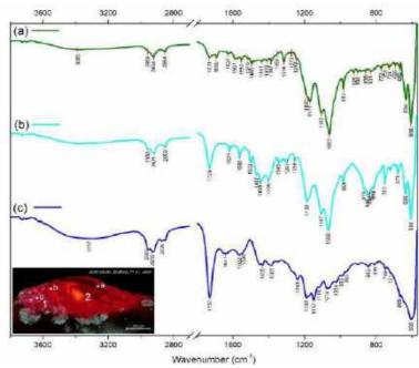
Fig. 7. μFTIR spectra from sample 21: (a) layer 2 contains alizarin crimson and Hansa yellow, among other pigments; (b) layer 2 contains Hansa red, among other pigments; (c) layer 1 contains brazilwood, alizarin crimson and starch
