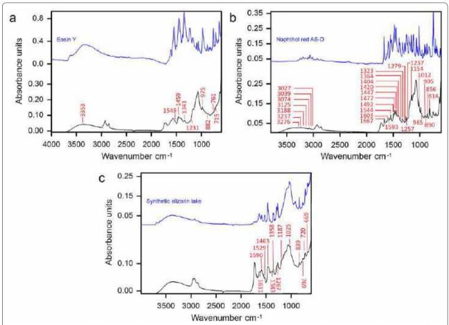
Fig. 16 a ATR-FTIR spectra of the red paint of sample 7 extracted from *Boats* with labelled marker peaks of organic red and reference spectra of eosin Y; b ATR-FTIR spectra of the red paint of sample 3 extracted from *Char Siew seller* with labelled marker peaks of organic red and reference spectra of naphthol red AS-D; c ATR-FTIR spectra of the red paint of sample 10 extracted from *Kampong scene* with labelled marker peaks of organic red and reference spectra of synthetic alizarin lake
