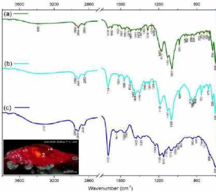
**Fig. 7.**  $\mu$ FTIR spectra from sample 21: (a) layer 2 contains alizarin crimson and Hansa yellow, among other pigments; (b) layer 2 contains Hansa red, among other pigments; (c) layer 1 contains brazilwood, alizarin crimson and starch
