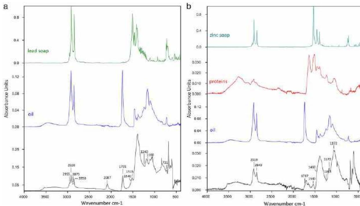
Fig. 11 ATR-FTIR spectra of grounds and reference samples of binders and metal soaps: **a** ground of type 1 from *Landscape in Switzerland*, with labelled marker peaks of oil and lead soap, peak 2087 indicates Prussian blue originating from the paint layer; **b** ground of type 2 from *Breakfast* with labelled marker peaks of proteins, oil and zinc soap
