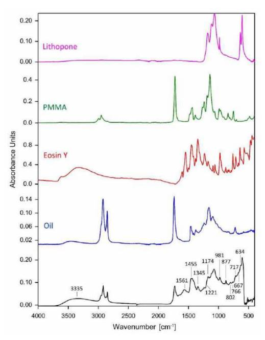
**Figure 13.** ATR-FTIR spectra of red paint from sample 29, taken from the *Boat near the cliff*, with labelled marker peaks of organic red and spectra of reference samples, identifying oil, eosin Y, acrylic resin, and lithopone.
