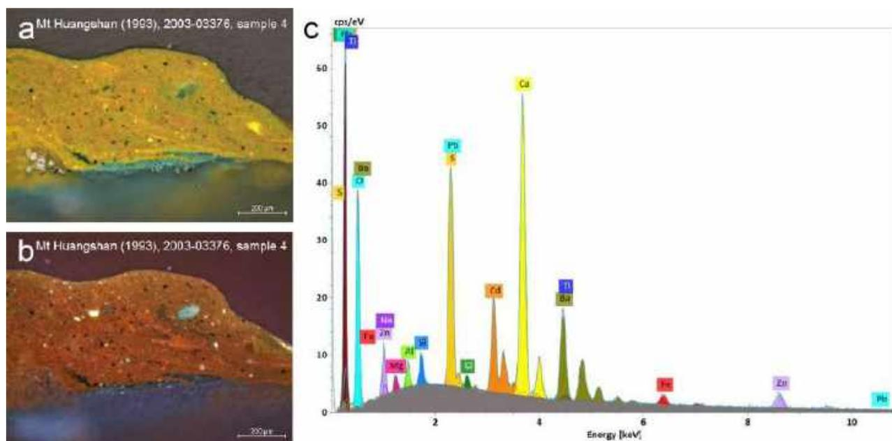
**Figure 12.** Optical microscopy images of the paint cross-section of sample 4, extracted from *Mount Huangshan*, 1993, photographed in: (a) VIS and (b) UV. The corresponding SEM-EDS spectra of the yellow paint (c). Red fluorescence of yellow paint and strong Cd and S signals combined with Ba and Zn suggests the use of cadmium yellow or cadmpone or zinc-modified light cadmium yellow.
