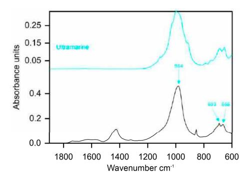
**Figure 7.** ATR–FTIR spectra derived from the blue paint of sample 6, collected from *Countryside in China*, 1933, with labelled marker peaks of ultramarine and reference spectra of the same pigment.
