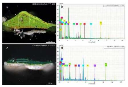
Fig. 5. Cross-sections and corresponding SEM-EDS spectra of green layers from samples 7 (a, b) and 3 (c, d). The SEM-EDS quantitative elemental analysis shows that the intensity of the green colour in both samples is determined by the presence of chrome yellow and viridian rather than the emerald green. The cross-section of sample 7 shows no evidence of an intermediate ground layer between the two painted compositions (layers 2 and 3)
