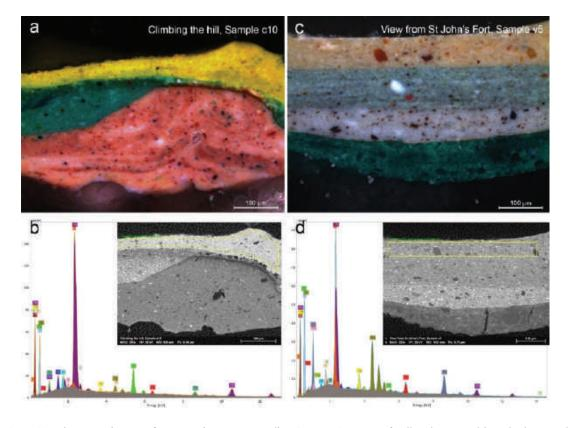
Figure 11. Microscopy images of cross-sections, corresponding SEM-EDS spectra of yellow layers, and inset backscattered electron (BSE) images with marked areas of analyses from sample c10 extracted from *Climbing the hill* (a, b), and from sample v5 extracted from *View from St. John's Fort* (c, d).
