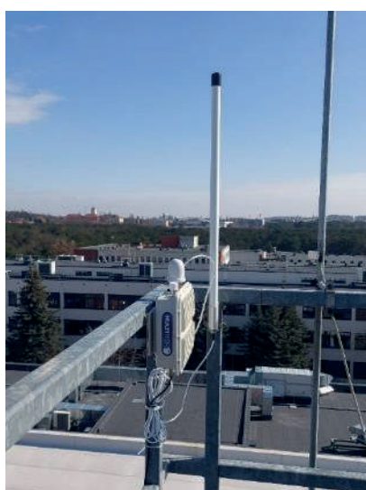
Fig. 4. External communication gateway of the LoRaWAN network with 34 cm (left) and 82 cm (right) antennas. Source: Authors' own elaboration.
