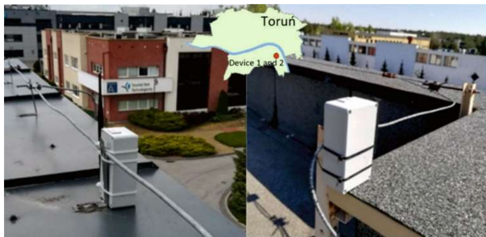
Figure 5. Automatic device (1 and 2) measuring the brightness of the sky, placed on one of the buildings in TARR (photo by Mieczysław Kunz).
