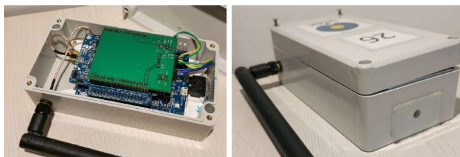
Figure 6. Pictures of the developed LoRa light measurement device (photo by Dominika Karpińska).
