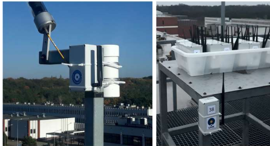
Figure 12. Pictures of the LoRa light measuring device deployed at outdoor locations (photo by Mieczysław Kunz).
