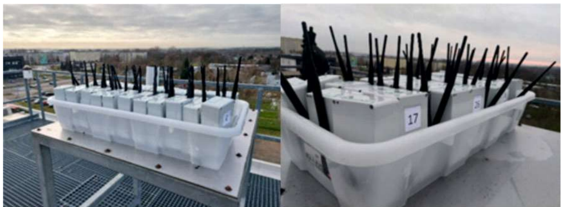
Figure 9. Test the cloud of 35 devices for measuring the sky brightness in winter 2020 on the terrace of the NCU Meteorological Observatory in Toruń (Poland) (photo by Mieczysław Kunz).
