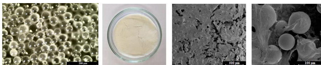
Fig.7. Polylactide microparticles and ALG/GEL/G(1%)/L(3.4%)+MPs matrix containing 2% sodium alginate (ALG), 1% gelatin (GEL), 1% glycerin (G), 3.4% oil phase (L): 2.4% oil from cotton seeds and 1% beeswax, and 6% microparticles (MPs) [H9]
